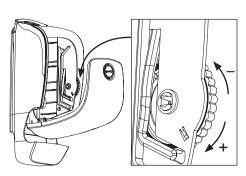
Roll Brake Settings Turn upwards to decrease roll breaking
